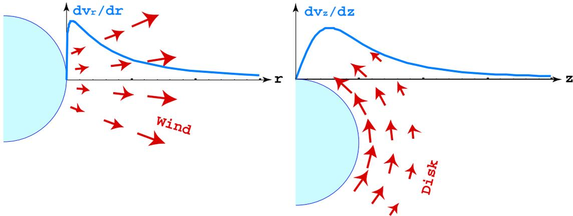
**Figure 1.** Comparison of the radial velocity gradient,  $dv_r/dr$ , of a radial stellar wind outflow with the line-of-sight gradient,  $dv_z/dz$ , along a ray direction  $z$  that is *tangent* to the stellar limb and passing through an orbiting Keplerian disk. The units of the gradient are arbitrary, but the relative scaling is accurate for the case in which the terminal velocity of the wind is the same as the near-surface orbital velocity of the disk.
